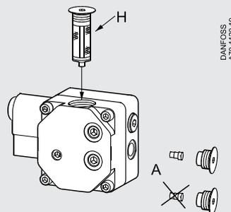
2-pipe operation: screw fitted
